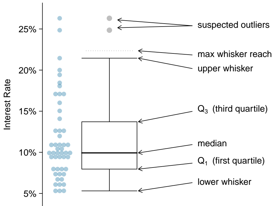
Figure 2.10: A vertical dot plot, where points have been horizontally stacked, next to a labeled box plot for the interest rates of the 50 loans.
